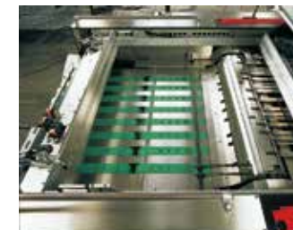
Synchronized belt speed to SPS® dryer sheet transition without flutter and friction.
